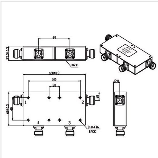
RF Solution offer a wide selection of Dual Junction Circulator for global customers. THH12060EN is a Dual Junction Circulator in Frequency Range of 80-230 MHz. It is made of high quality materials under a high standard, the Bandwidth Max of this product is 30%, Insertion Loss Max is 2.2 dB and Isolation Min is 36.0 dB. The component has a good working performance and stability, it is ideal for handling a Forward Power of 150 W.
